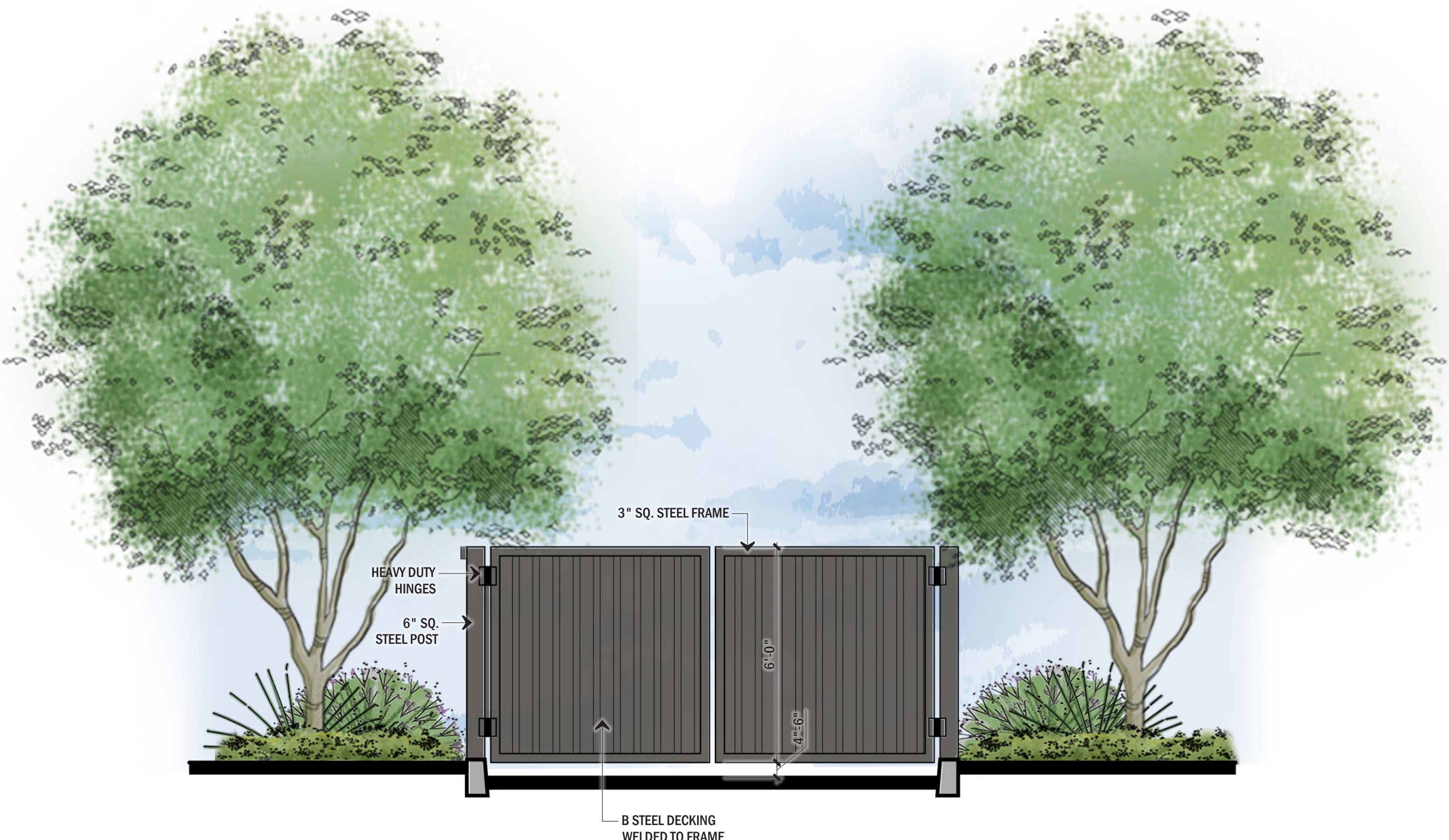
1 TRASH ENCLOSURE GATE
