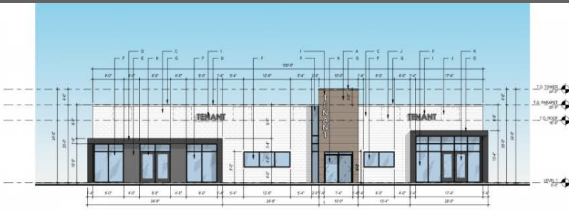
1 FRONT ELEVATION BUILDING B.C 1/8" = 1'-0"
