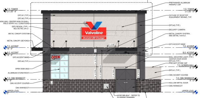
2 EXTERIOR ELEVATION (OVERALL EAST FACADE) SCALE: 1/8" = 1'-0"
