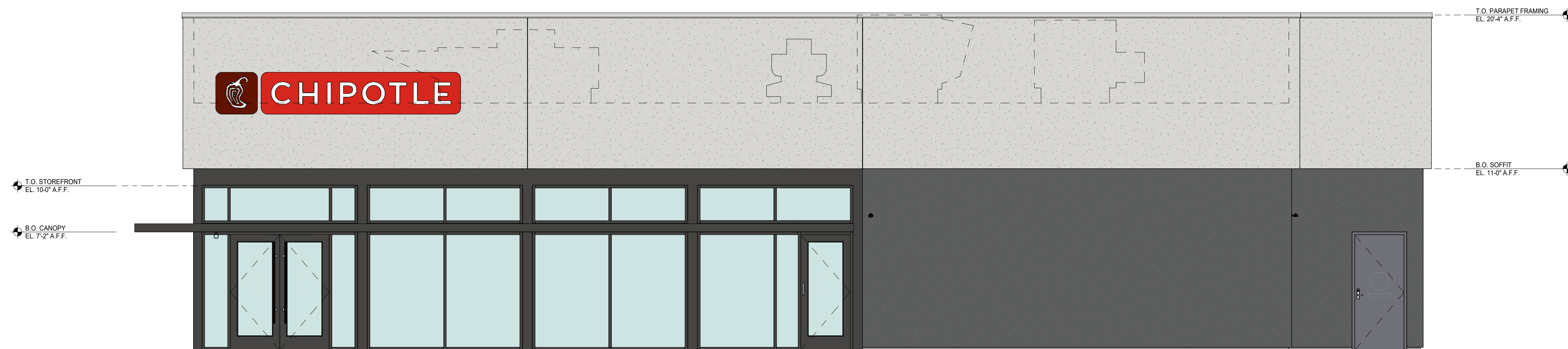
1 EXTERIOR ELEVATION - WEST 1/4" = 1'-0"
