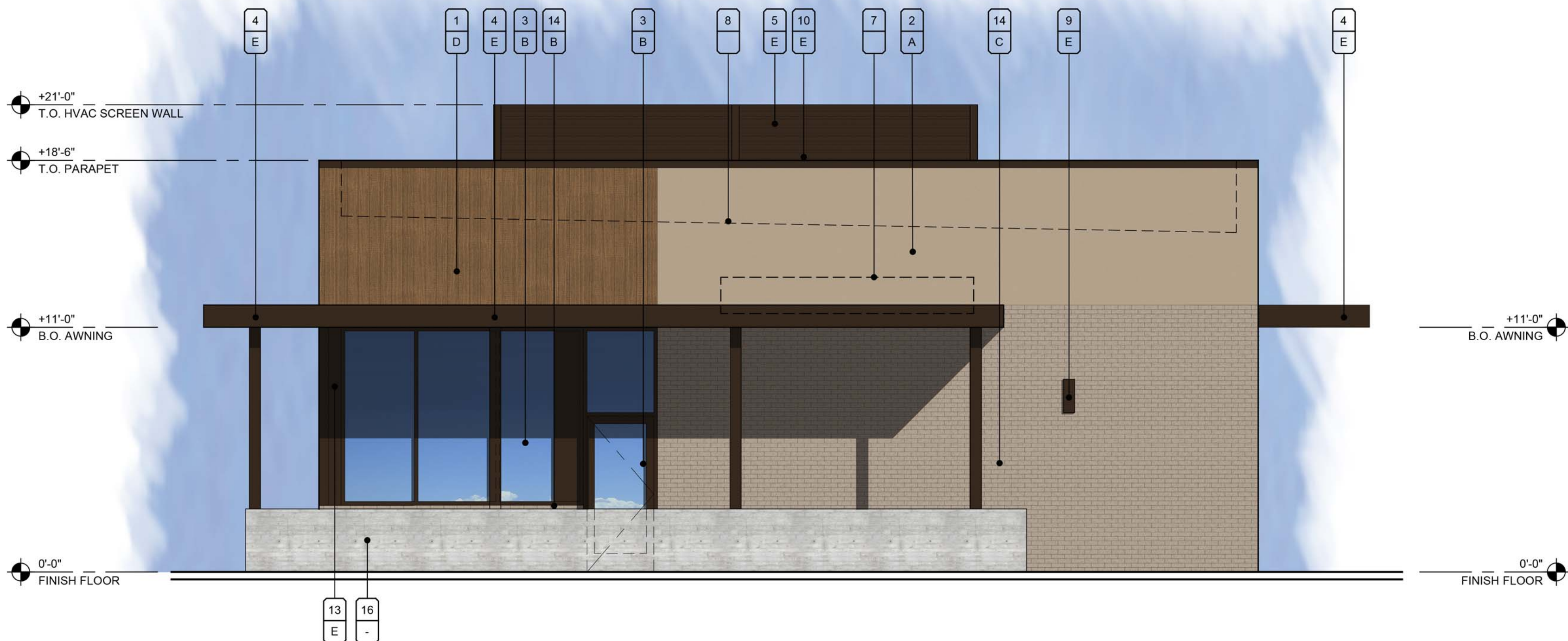
4 NORTH ELEVATION SCALE: 1/4"=1'-0"
