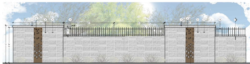
3 6' PARTIAL VIEW FENCE SCALE: 1/2" = 1'-0"
