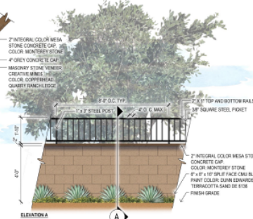
4 Combo Wall / View Fence SCALE: 1/2"=1'-0"
