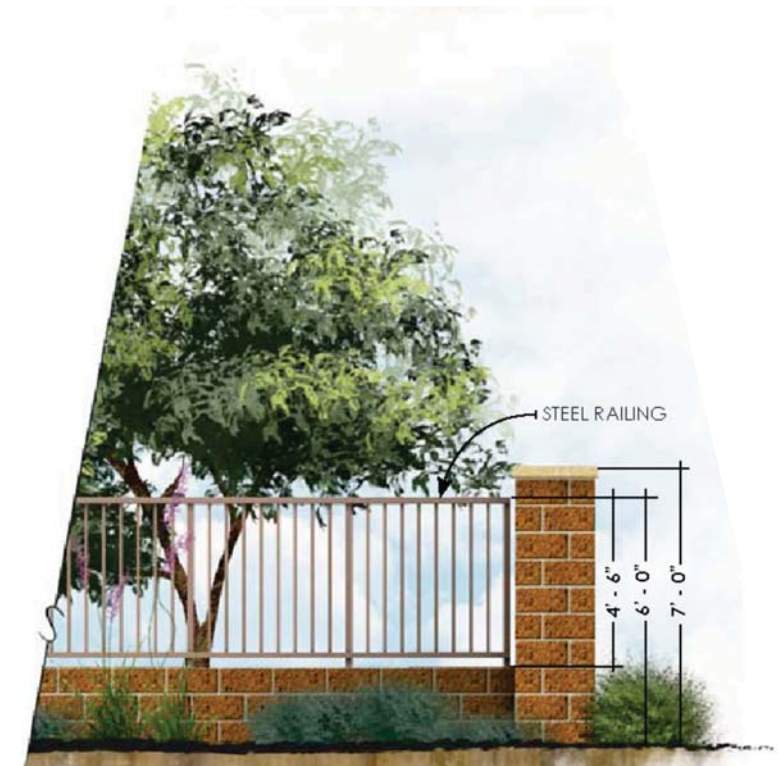
5 FULL VIEW WALL ELEVATION NTS
