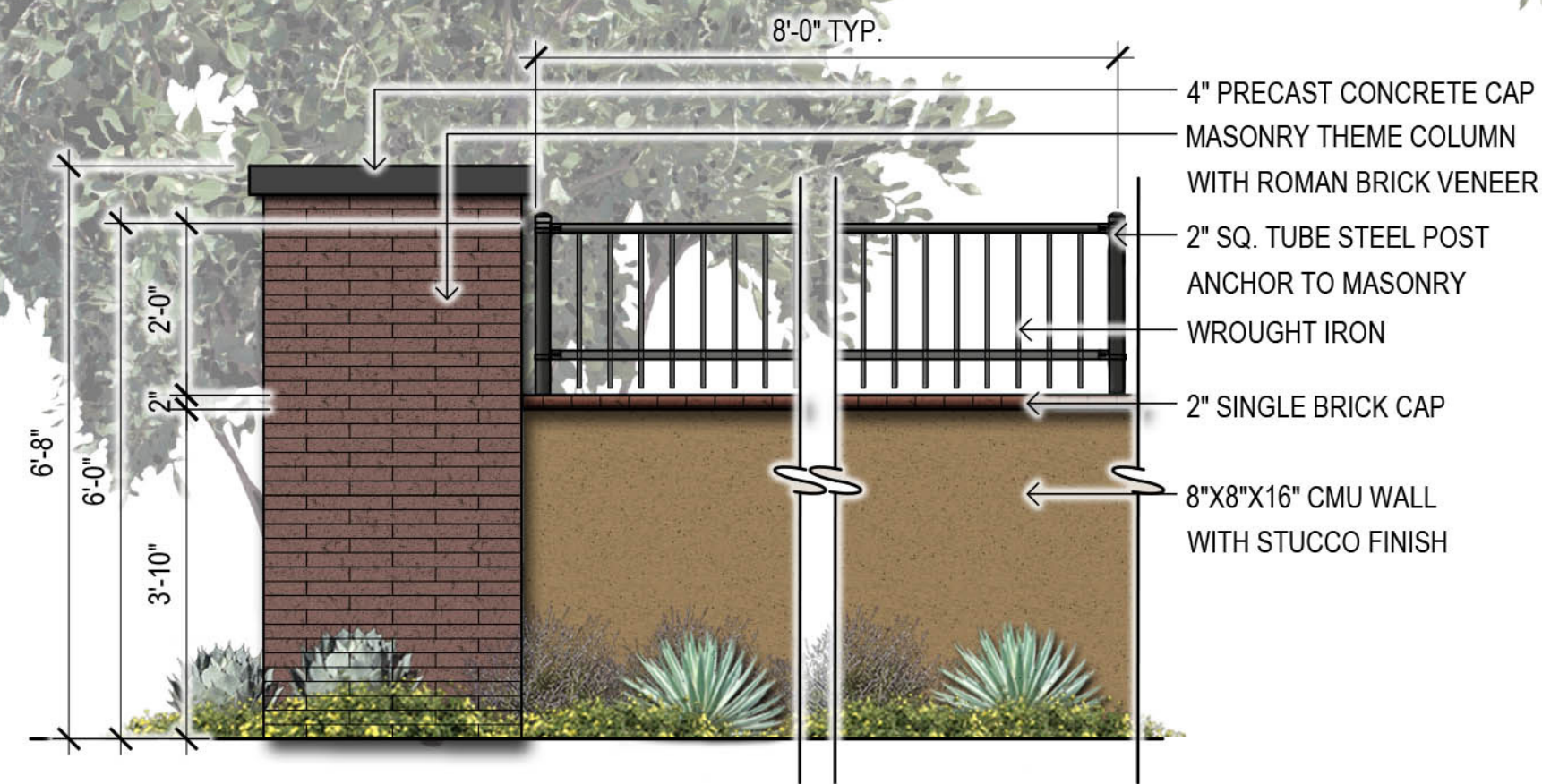
2 Combo View Wall - 2' View / 4' Solid SCALE: 1/2"=1'-0"
