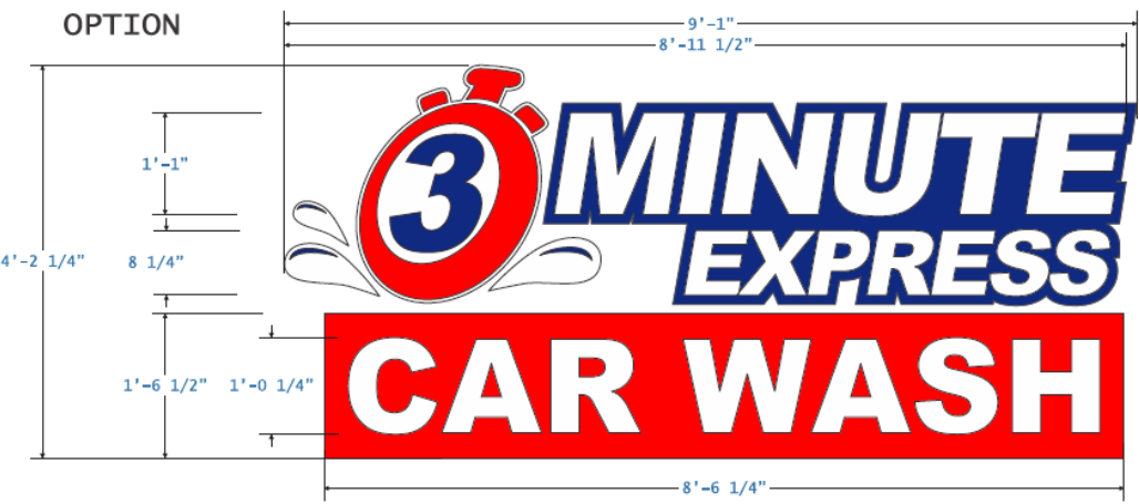
ILLUMINATED FACE AND HALO DISPLAY SCALE: 3/4" = 1'-0" 37.45 sq.ft.
