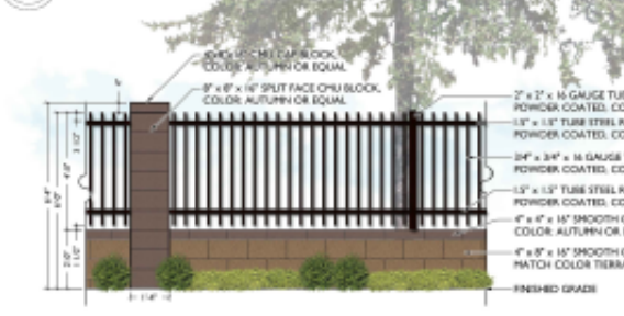
4 PARTIAL VIEW WALL TYPE B WITH 'COLUMN A' Scale: 1/2" = 1'-0"
