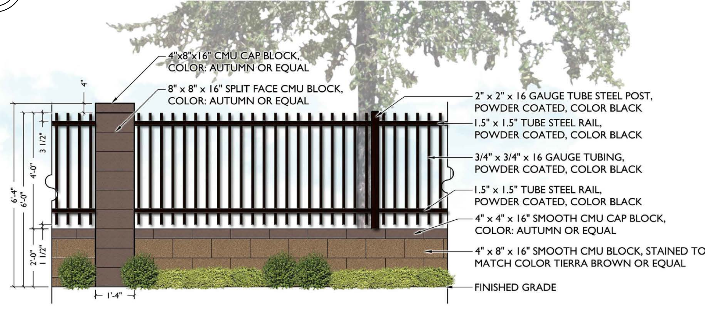
4 PARTIAL VIEW WALL TYPE B WITH 'COLUMN A' Scale: 1/2" = 1'-0"
