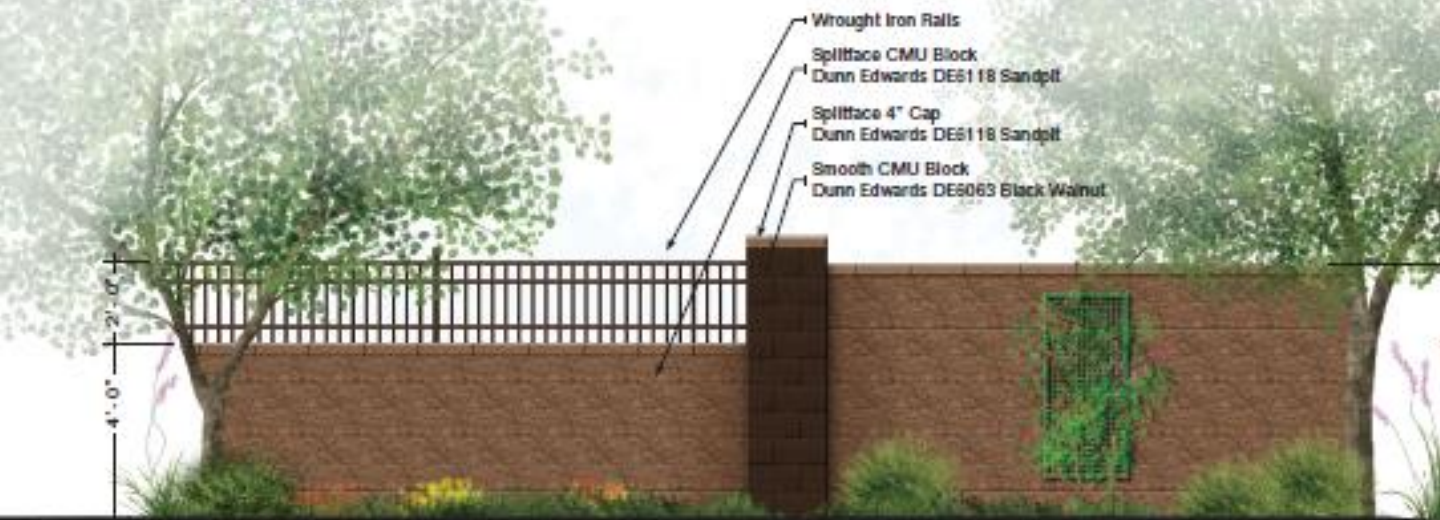
Partial View Wall
