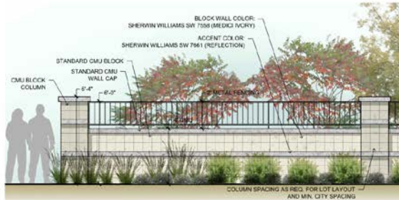
PARTIAL VIEW WALL
