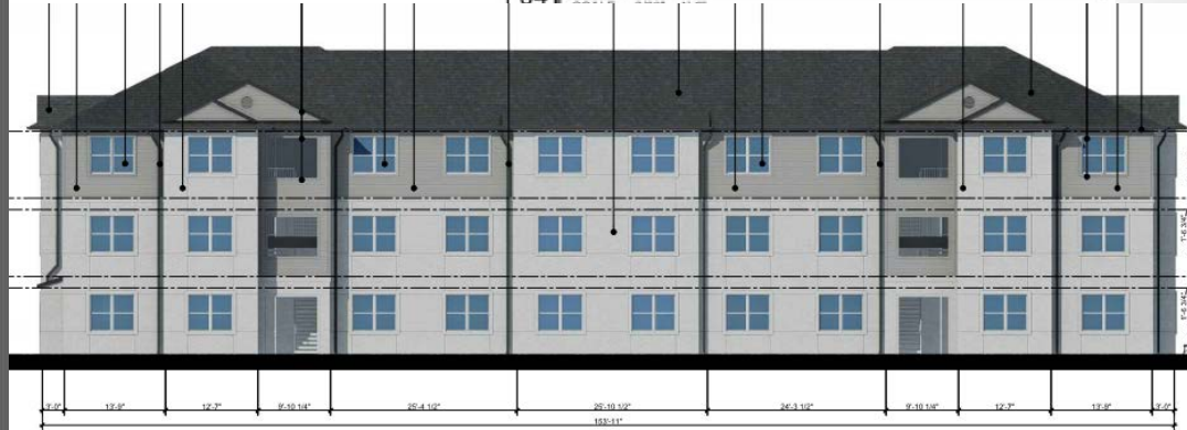
01 BUILDING TYPE II - FRONT ELEVATION
