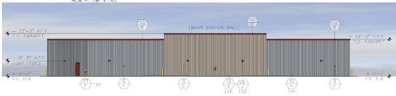
NORTHSIDE ELEVATION - BUILDING 'F' (WASH STATION) SCALE: 1/8" = 1'-0"
