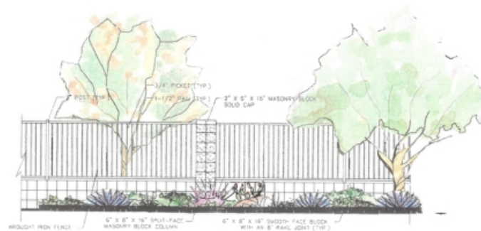
VIEW FENCE/WALL ELEVATION A00.001 TO 004 00.00
